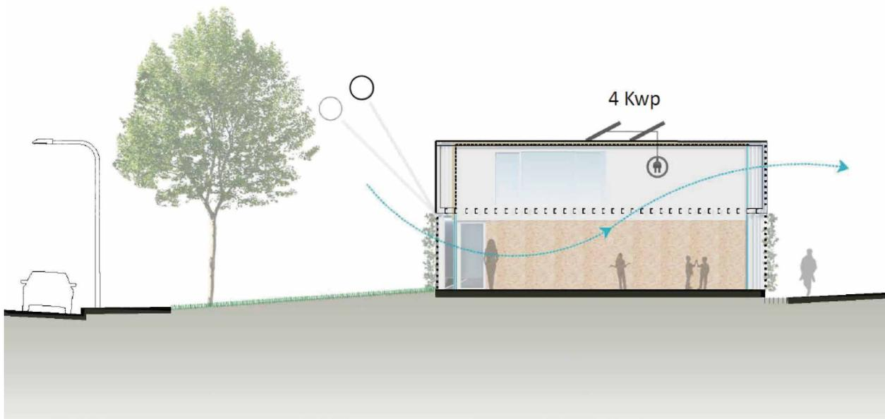
Figure 70. Profile of the center with indication of cross-ventilation and renewable energy production. Image provided by AMB.
