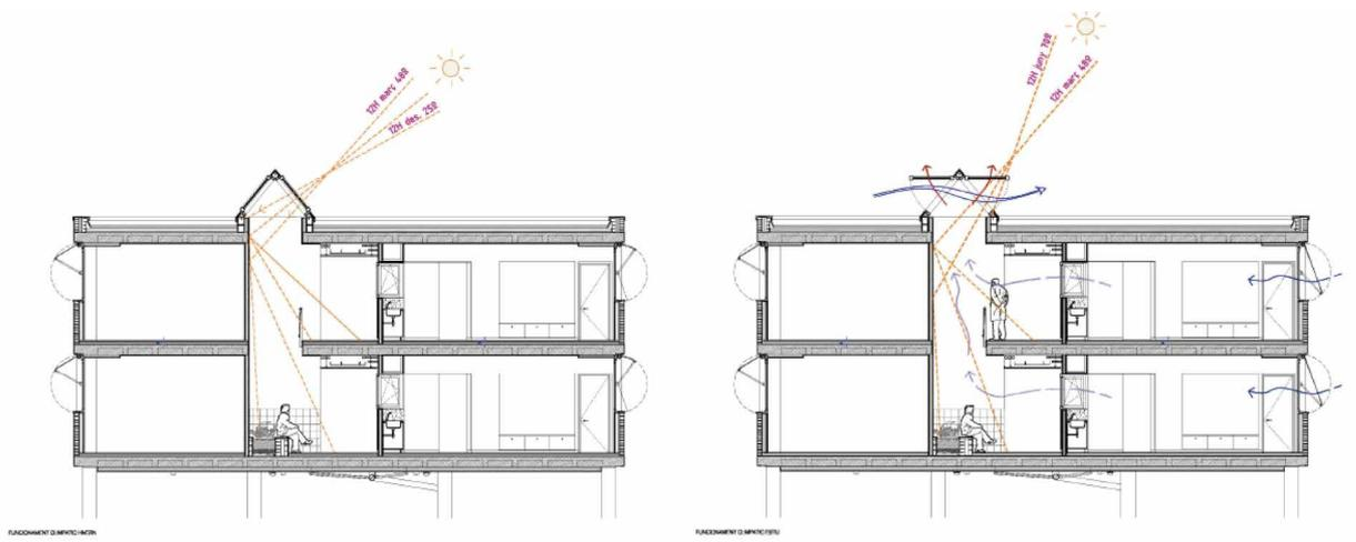
Figure 30. Profile of the Carrer El Pla showing vertical openings for ventilation. Image provided by AMB.
