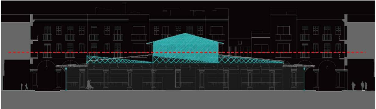
Figure 68. Proposed market building design, with eliminated middle section volume colored in blue. Image provided by AMB.
