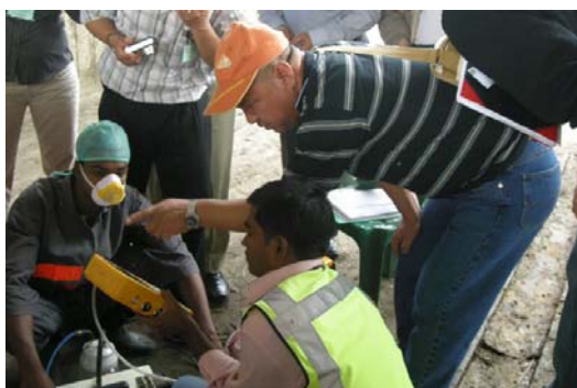
Local compost plant workers show how the oxygen and methane levels of the waste are measured. Detailed records are kept to comply with the regulations necessary to gain carbon credits.
